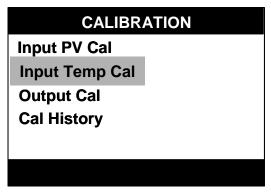
Use the ▲▼ keys to highlight the "Input Temp Cal" selection.
